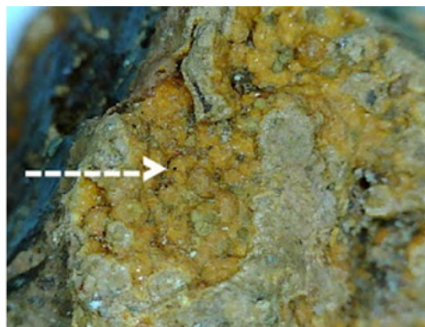
Spherical encrustation of tan to orange hidalgoite composed of micro crystals; each sphere ranges from .3-.5 mm. Specimen is from Gold Hill, Utah. Photomicrograph by Mike Nelson.
